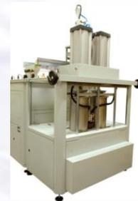
Hybrid version incorporates press-out modules for high viscosity materials
